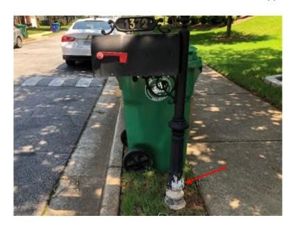
The posts have a very long life if not hit by a vehicle. At the time of the original installation the Association opted to not have the mailbox posts mounted to the concrete bases, so the paint at the bottom of many of the posts have been damaged by string trimmers. Repainting of the posts and the mailboxes is included in the **Gazebo** category along with the metal fencing and entrance gates every six years.
